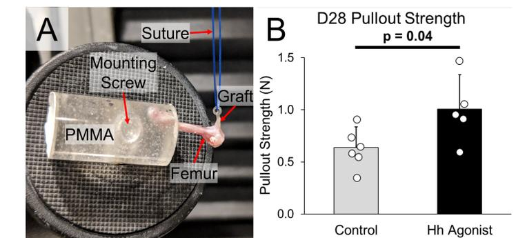
**Fig. 5: Hh agonist treatment yielded improved tunnel pullout strength 28 days post-surgery.** Femurs were mounted in PMMA while a suture was attached to the washer on the femur as well as the actuator of the testing machine (A). The washer was pulled until the graft was removed from the tunnel. Agonist-treatment yielded a 60% greater pullout strength than PBS controls (p = 0.04, B).
